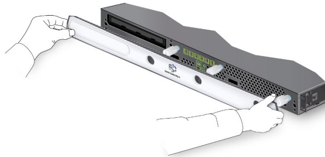
Figure 5 Removing Front Panel of an M500 Player
