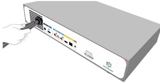
Figure 4 Vacuuming Alto and Cinema One Air Outlet Grille
