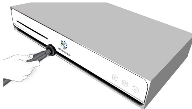
Figure 3 Vacuuming Alto and Cinema One Air Inlet
