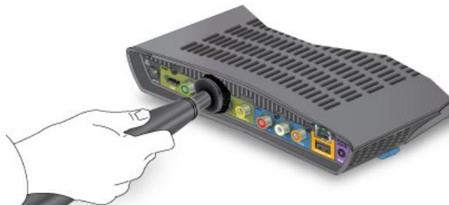
Figure 14 Vacuuming M300 Player Air Outlet Grille
