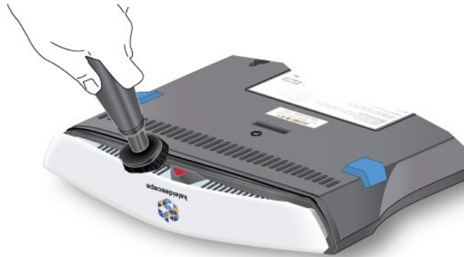
Figure 13 Vacuuming M300 Player Air Inlet Grilles
