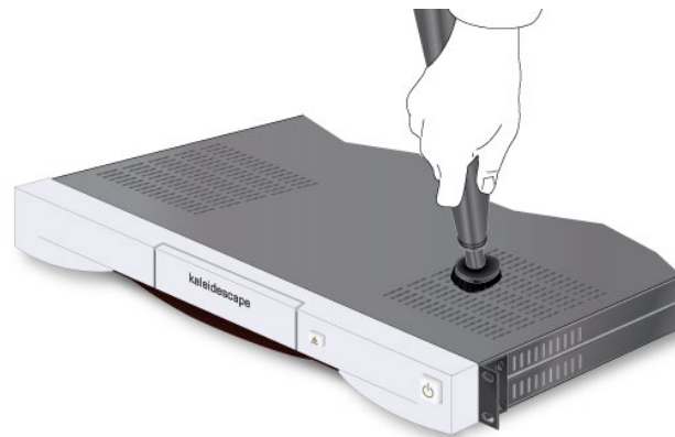
Figure 19 Vacuuming Reader Top Grilles
