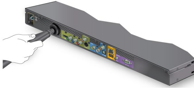
Figure 9 Vacuuming M500 Player Air Outlet Area
