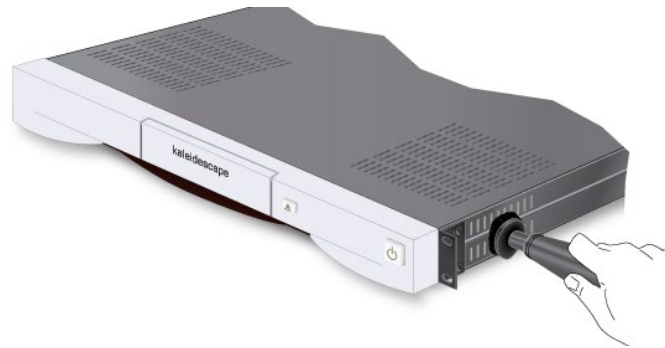
Figure 18 Vacuuming Reader Side Grilles
