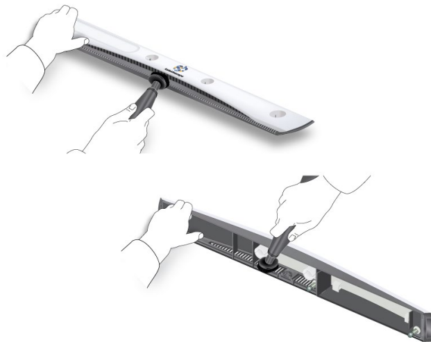
Figure 7 Vacuuming M500 Player Air Intake Areas
