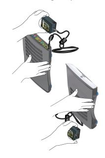
Verify that there is adequate airflow around the player, allowing for hot air exhaust [1 in. (2.5 cm) in front and 2 in. (5 cm) in back minimum].
