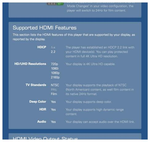
This section details the copy protection, resolution, TV standard and color capabilities of the display, and indicates whether audio is accepted by the display. Note that it is normal for HDCP 1.x to be rendered with a line through it when HDCP 2.2 is supported, because of how Strato C detects HDCP. When HDCP 2.2 is active, Strato C cannot detect whether the display also supports HDCP 1.x.
