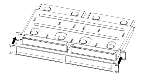
5. The bottom flange on the fascia will go on the outside of the shelf. This panel is not firmly attached until the shelf is installed in the rack.
