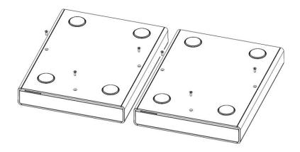
3. Place the rack shelf over the units. Note the appropriate sets of holes to be used in the diagram below. Orient the shelf so the mounting holes are lined up with the holes in the players where the screws were removed. Move the shelf into position as required by the installation. In the frontmost position the player faces will protrude by 3/4" (recommended). In the rearmost position, the faces of the players are flush with the front of the rack ears. Install the saved screws:
