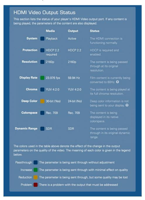
The example above shows Strato C playing 4K Ultra HD film content on the same projector. Strato C has been set to minimize display mode changes, so it is converting the 24 fps film content to 60 fps. At 60 fps, this projector is not
