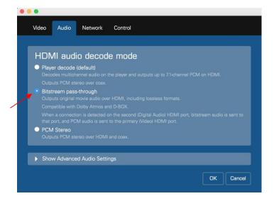
Bitstream audio can be output from one HDMI port at a time. Strato C sends the bitstream audio to the DIGITAL AUDIO HDMI port if it detects a connection on that port. Otherwise, it sends the bitstream audio to the VIDEO HDMI port.
