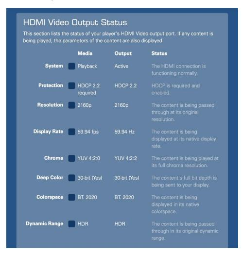
In the example above, Strato C is taking full advantage of an 18 Gbps connection to play a 60 fps 4K HDR movie on a display that supports the maximum possible HDMI 2.0a connection. Note how HDR content shows differences in the Colorspace and Dynamic Range lines compared to the examples above.
