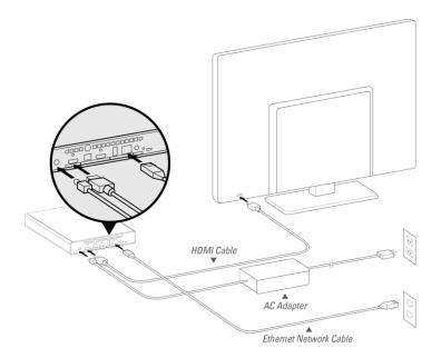
Connect network, audio and video cables before connecting the AC adapter.
