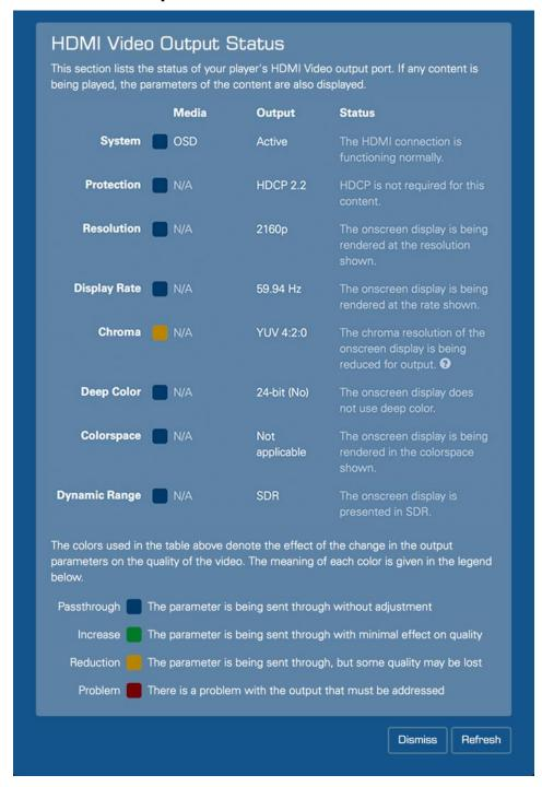
This section shows the output status of the HDMI port, as of when the window was opened or refreshed. It works when displaying the onscreen display, and while playing content, so you can use it to confirm that 4K Ultra HD content is being displayed at full resolution, that 1080p content is being up-scaled, and that the expected frame rates and color information are being output.
