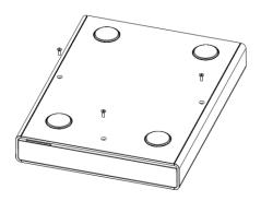
3. Place the rack shelf centered over the unit. Note the appropriate sets of holes to be used in the diagram below. Orient the shelf so the mounting holes are lined up with the holes in the player where the screws were removed. Move the shelf into position as required by the installation. In the frontmost position the player face will protrude by 3/4" (recommended). In the rearmost position, the face of the player is flush with the front of the rack ears. Install the saved screws:
