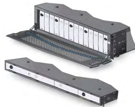
Figure 9 Staggering disk cartridges with blank cartridges reduces disk temperatures and can increase the lifespan of the drives
