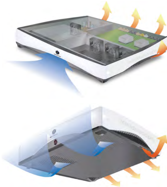
Figure 12 Kaleidescape Mini Systems intake cool air from the front and bottom, and exhaust hot air through vents located on the back and right side of the chassis
