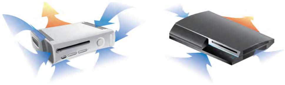
Figure 6 Gaming consoles typically intake cool air from many surfaces and exhaust hot air through vents located on the back of the chassis
