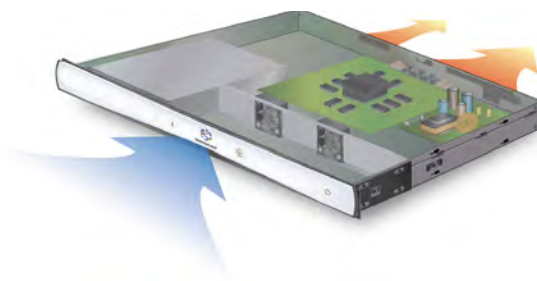
Figure 10 Kaleidescape players intake cool air from the front and exhaust hot air through vents located on the back of the chassis
