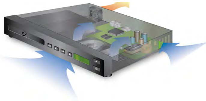
Figure 2 DVR and Blu-ray players typically intake cool air from the bottom and sides and exhaust hot air through vents located on the back of the chassis
